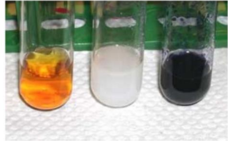
Left to right: Lugol's iodine, starch solution, starch solution with iodine.
